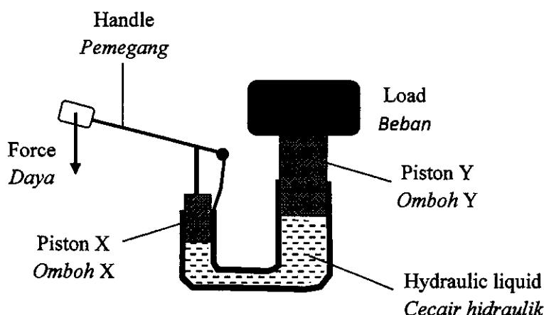
The jack can lift a heavier load using the same force by
