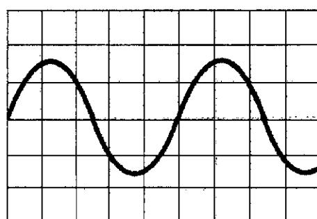
The Y-gain and the time-base are set at 3 volt / division and 5 ms / division respectively. What is the peak voltage and the frequency of the alternating current supply that connected to the C.R.O?
