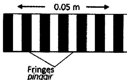
The distance between double slit and screen is 1 m and the wavelength of light is given as  $5 \times 10^{-7}$  m. What is the distance between two slits?
